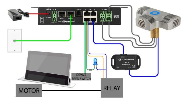
Pictured above, the CDT100 MkII is using output Pin #2 and the 12V supply from Pin #4 to trigger the Motor relay. The limit switch is sending a feedback via an input Pin #5 by grounding to Pin #3 and the LED is powered by Pin #4 and turned on by the internal grounding of Pin #6.
