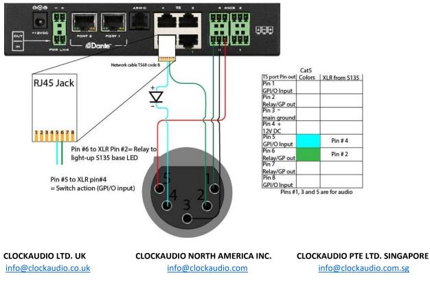
The image above shows the connector of an S135 connected to input Pin #5 for sending the pulse of the 'button press' and output Pin #6 to light up the LED on the base.
